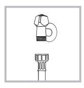
1. Connect the inlet hose by screwing it to a cold water tap using a 3/4 gas threaded connection (see figure). Before performing the connection, allow the water to run freely until it is perfectly clear.
