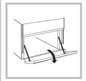
There is a compartment underneath the oven that may be used to store oven accessories or deep dishes. To open the door pull it downwards ( see figure ).
