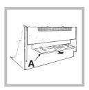
To remove the sliding protection remove the screw S (see figure). To replace it, lock it in place with the screw S.
