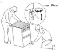
**CAUTION:** Some soft floor coverings may get damaged if the cooker is not moved carefully. Badly leveled device may increase condensation.
