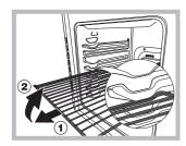
WARNING! The oven is provided with a stop system to extract the racks and prevent them from coming out of the oven.(1) As shown in the drawing, to extract them completely, simply lift the racks, holding them on the front part, and pull (2).
