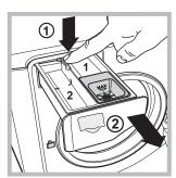
To remove the drawer, press lever (1) and pull the drawer outwards (2) (see figure).
