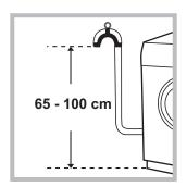
Connect the drain hose to drain duct piping or a wall drain located between 65 and 100 cm above the floor, making sure it is not bent at all.
