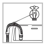
Alternatively, place the drain hose over the edge of a washbasin or bathtub, by fastening the guide (which can be purchased at the technical assistance centre) to the tap (see figure). The free end of the
