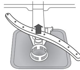
The lower spray arm may be removed by pulling it upwards.
