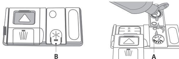
1. Open the dispenser **B** by pressing and pulling up the tab on the lid.
