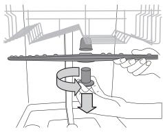
To remove the upper spray arm, turn the plastic locking ring in an anticlockwise direction. The upper spray arm should be replaced so that the side with the greater number of holes is facing upwards.
