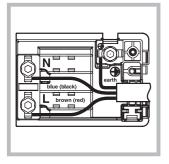
2 Loosen the cable clamp screw and remove it, using a screwdriver as a lever (see figure).
