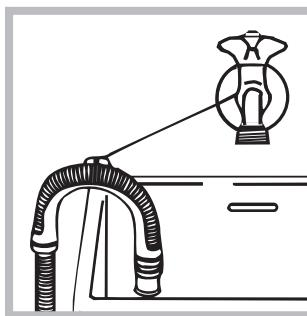
Alternatively, place the drain hose over the edge of a washbasin or bathtub, by fastening the guide (which can be purchased at the technical assistance centre) to the tap (see figure). The free end of the hose should not be
