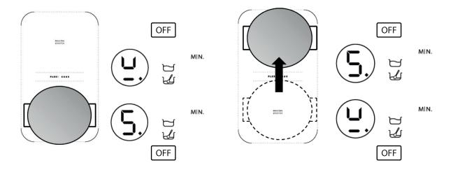
It is also possible to operate the Flexi cook area as two independent cooking zones, using the corresponding button of the single zone. Place the pot in the center of the single zone and adjust the power level with the slide touchscreen.
