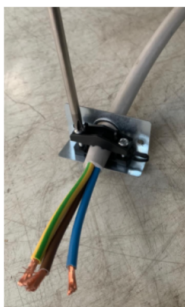
Fix power cord to the plastic holder.
