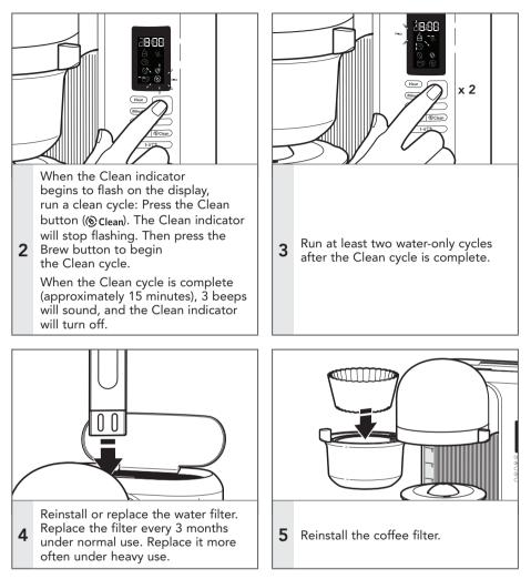
**IMPORTANT:** The Clean cycle can be completed at regular intervals, if desired, without the Clean indicator needing to light up. Follow these directions to clean the Coffee Maker whenever desired.
