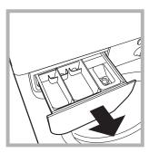
Remove the dispenser by raising it and pulling it out (see figure). Wash it under running water; this operation should be repeated frequently.
