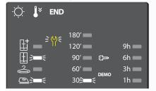
The presence of wrench symbol signals a malfunction. Carry out the operations described. Switch the dryer off and unplug it. Open the door immediately and pull landry out, to allow the heat to dissipate. Wait for about one hour. Reconnect the dryer to the power supply, load the laundry and restart the drying cycle.
