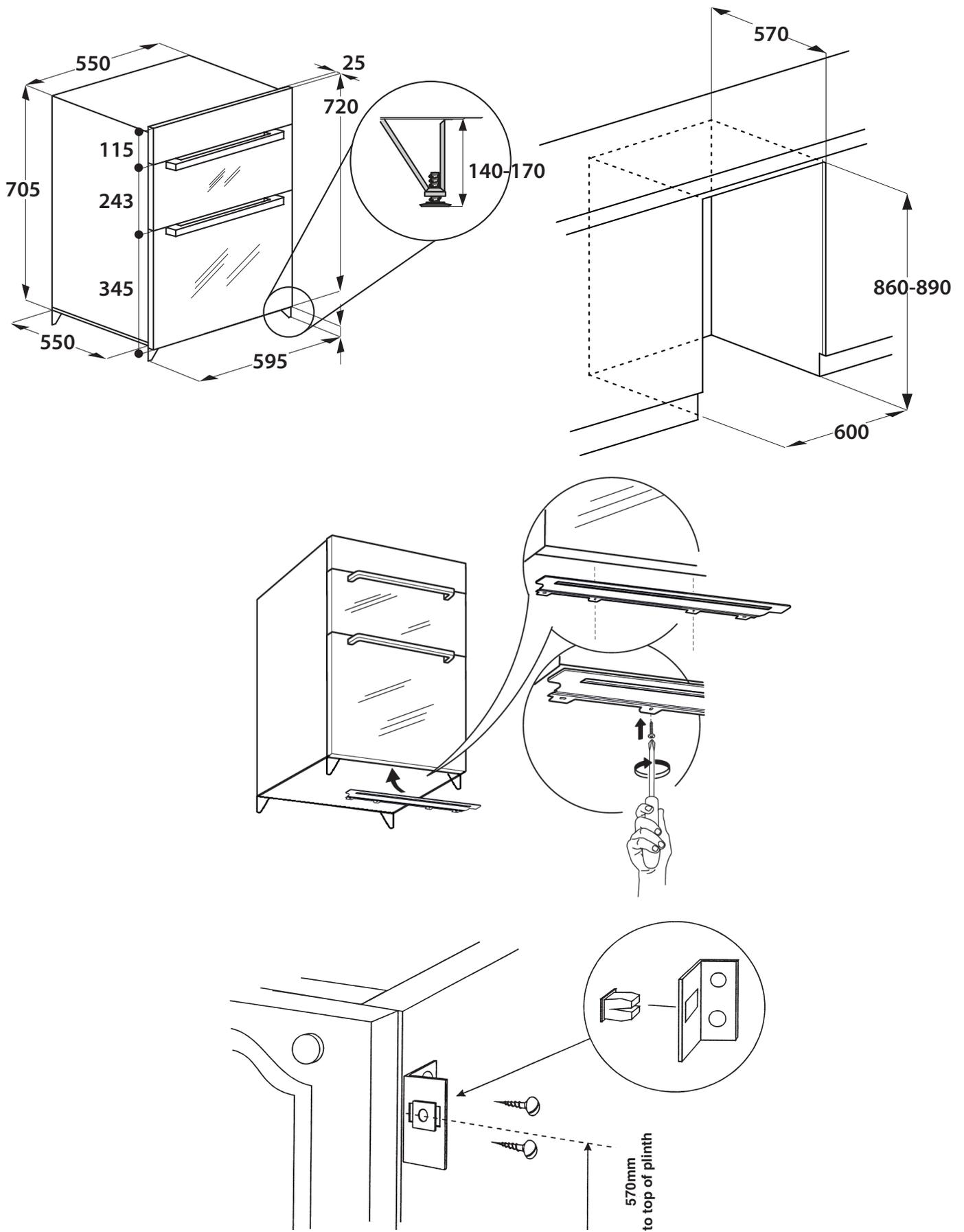
A minimum distance of 25mm should be maintained between the front face of the cabinet side and the front face of the plinth.
