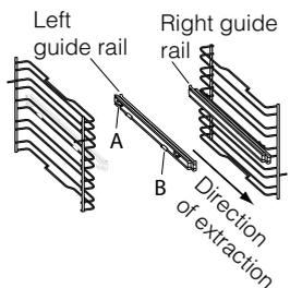
2. Choose which shelf to use with the sliding rack. Paying attention to the direction in which the sliding rack is to be extracted, position joint A and then joint B on the frame.
