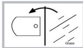
2. Turn the brackets so that the glass can be removed and cleaned at the sink (Fig. 1.).
