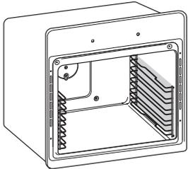
1. To remove the two side grilles, unscrew the screws from the catalytic panels.
