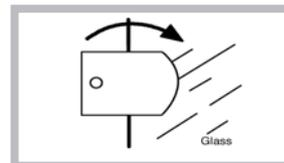
2. Turn the two securing brackets back to their original position to retain the glass and tighten the screws (Fig. 2.)
