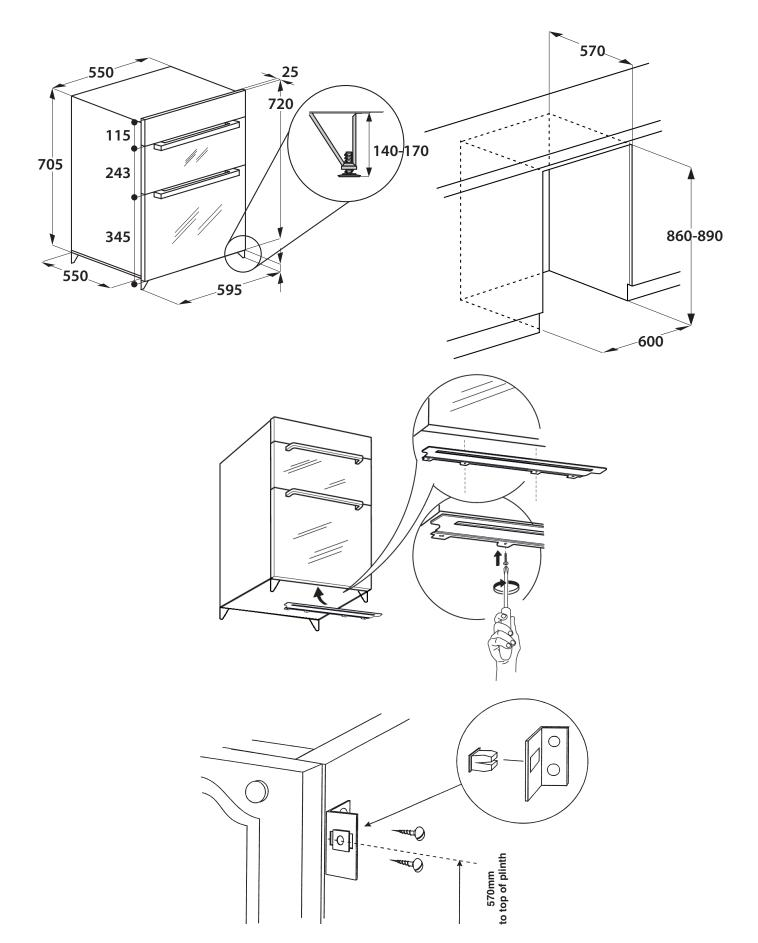
A minimum distance of 25mm should be maintained between the front face of the cabinet side and the front face of the plinth.
