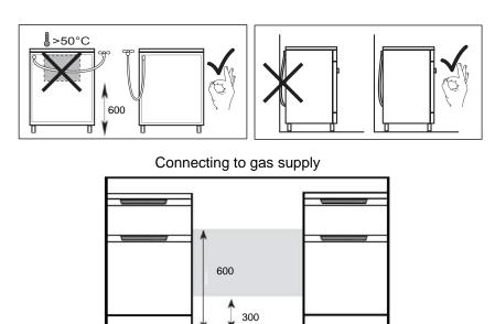
Gas hose connection point must be installed within the shaded area
