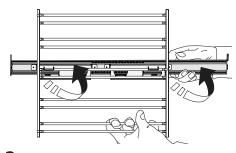
**3.** To reinstall the sliding guides, anchor the guide's upper clip to the shelf guide, then lower the other clip into position.
